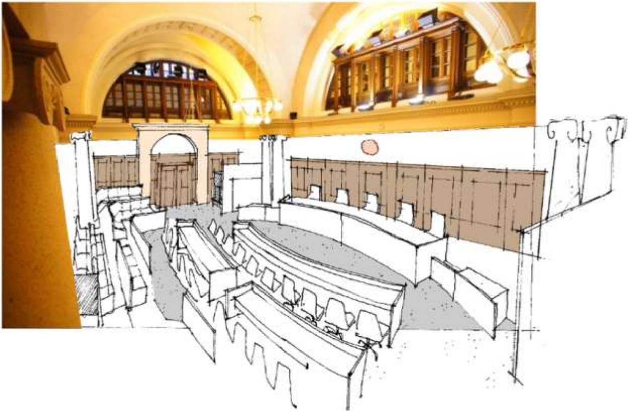
Image of the Large Court Room of the Court of Final Appeal converted from existing Chamber of the former Legislative Council
